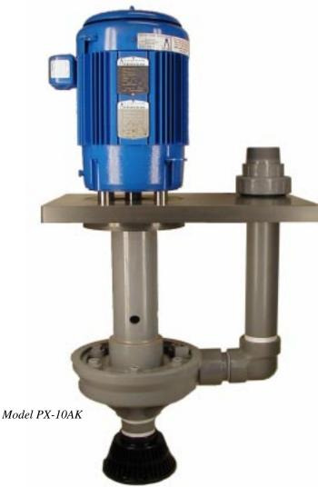
Our new Penguin extended vertical immersible pumps are simple in design, efficient in performance, and self-priming when immersed in solution. Constructed completely of CPVC with PTFE wear ring, or CPVC with PVDF impeller where in contact with the solution, this pump is suitable for pumping, agitating, filtering, or circulating acid and alkaline solutions, abrasive fluids, and other corrosive solutions up to 180 degrees F maximum temperature.
